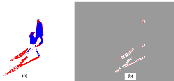
Figure 5: Poor shadow detection (a) producing unreliable line segments (b)
