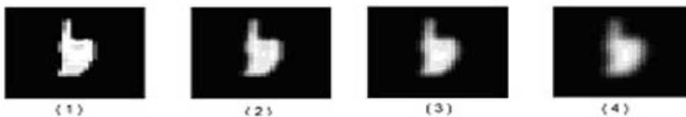
Figure 2. Images under different blurring factors: (1) is the original image, i.e. \sigma = 0 . From (1) to (4), the blurring factors are 0, 0.5, 1.0, 1.5 respectively.
