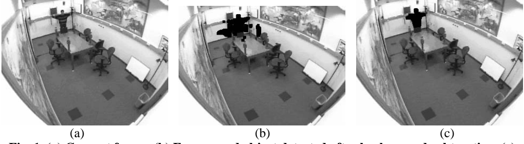
Fig. 1. (a) Current frame. (b) Foreground object detected after background subtraction. (c) Foreground object after background subtraction with shadow detection and removal.
