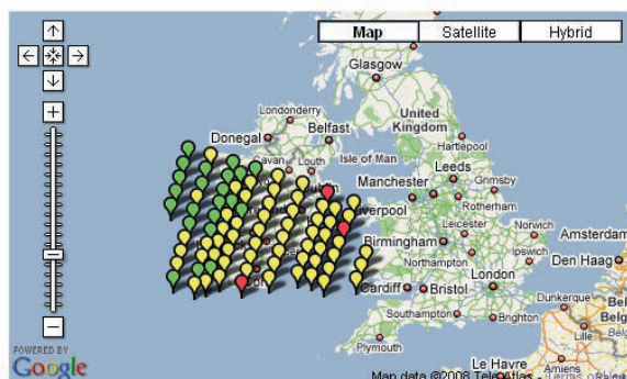
Figure 2: The SCIAMACHY instrument operates in three modes Nadir, Limb, and Occultation. For a single day the Nadir measurements do not cover all of Ireland (and the UK) and so data is typically built up over several weeks. For example, on this day although most of northern Ireland was not covered by the nadir measurement.
