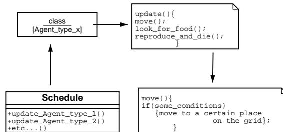
Figure 1: Schematic outline of a typical ABM with “closed” agents. The agents’ `update()` methods are called according to a schedule. The update usually consist of a series of more basic actions to be taken, such as movement, uptake of food and reproduction and death. How exactly these actions are performed and under which conditions they are called may be variable—within some pre-defined limits—which enables evolutionary agent adaptation.
