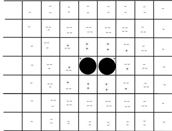
Figure 3: Overlapping potential fields superpose linearly.
