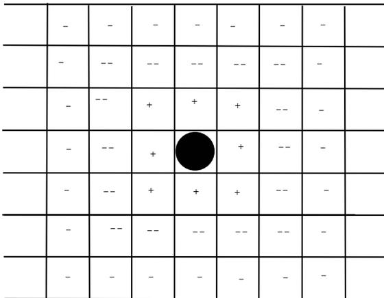
Figure 2: Potential field established by an isolated particle.
