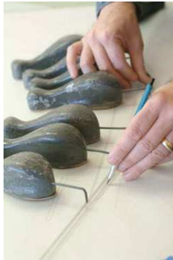
Figure 2.50: An example of how lead weights known as ducks can be used to generate a curved shape from a straight rod.
