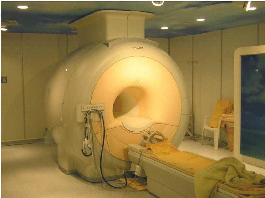
Figure 4.15: A three tesla Philips MRI scanner.
