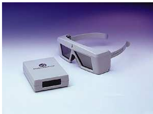
Figure 4.17: The CrystalEyes LCD shutter glasses and remote control unit.
