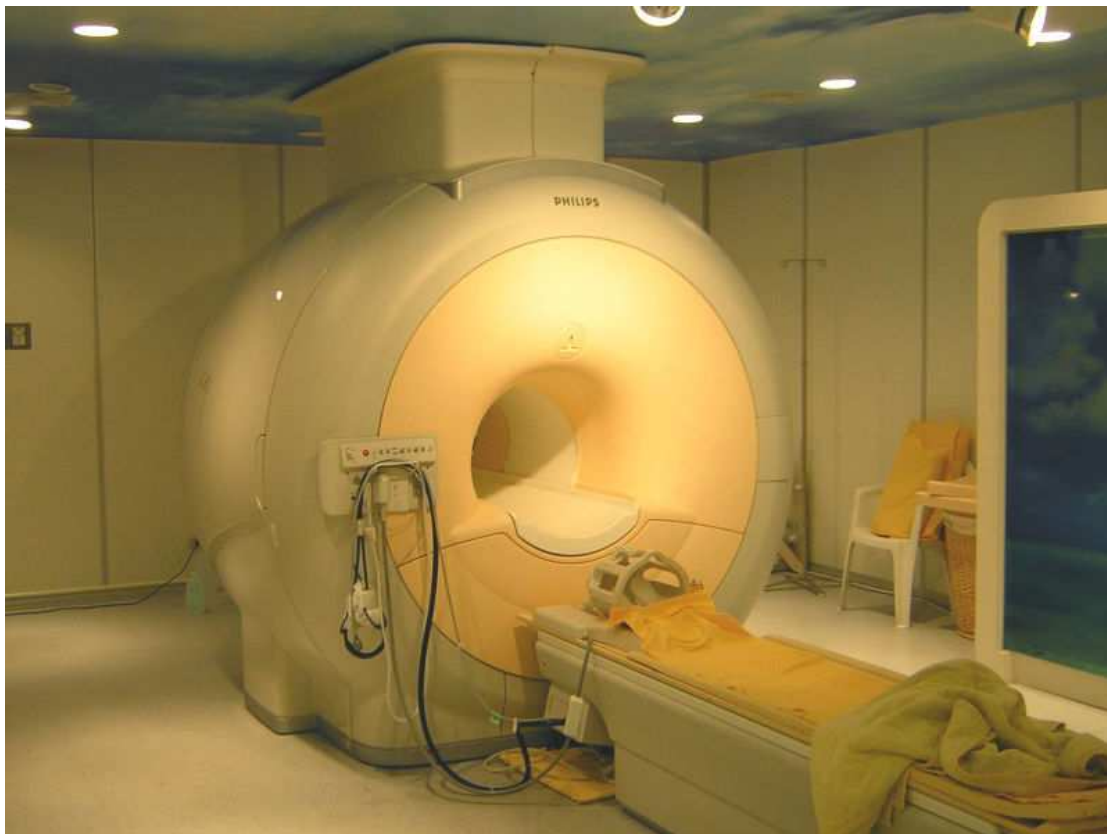
Figure 4.15: A three tesla Philips MRI scanner.
