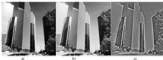
**Figure 3 :** Retinal pre-processing. The original image (a) is subject to a local adaptive compression by photoreceptors (b), then is high-pass filtered by the retinal circuits (c). Notice contrast equalization across the whole image.
