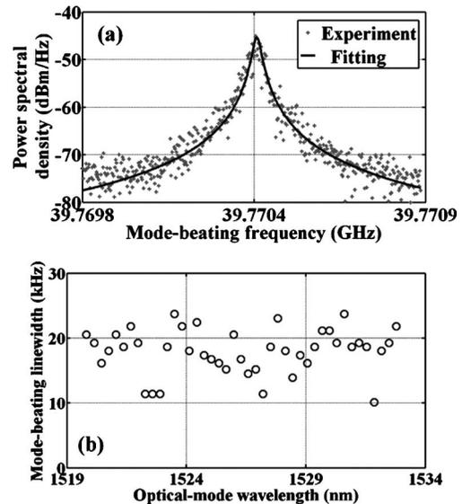
Fig. 3. (a) Typical mode-beating signal measured at the output of our QDash-MLLD at 350 mA and (b) mode-beating linewidth associated with each pair of optical modes as a function of the BPF central wavelength.
