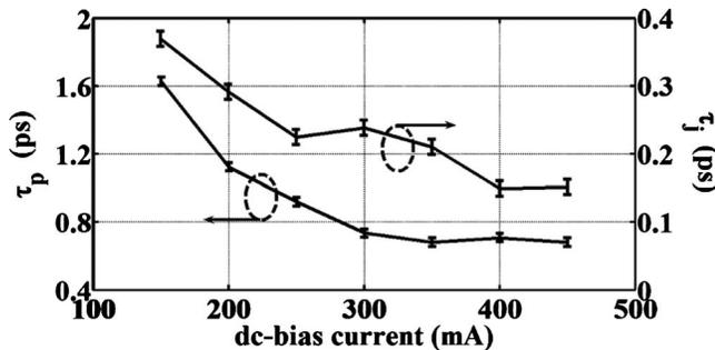
Fig. 4. Pulse width ( $\tau_p$ ) and timing jitter ( $\tau_j$ ) associated with the optically generated pulses in terms of the dc-bias current supplied to the DUT.
