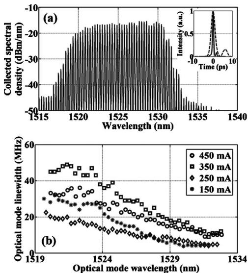
Fig. 2. (a) Typical optical spectrum collected from the QDash-MLLD at 350 mA and (b) mode linewidth measurements as a function of the bias current. In the inset, pulse profile at the output of the QDash-MLLD (dotted curve) and after passive compression (solid curve).
