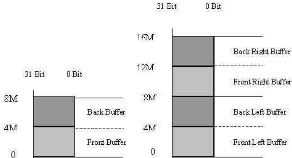
Figure 5. Double-buffered (left picture) and Quad-buffered (right picture) memory organisation
