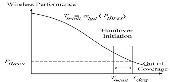
Figure 1. Handover Initiation Based on  $T_{deg}$
