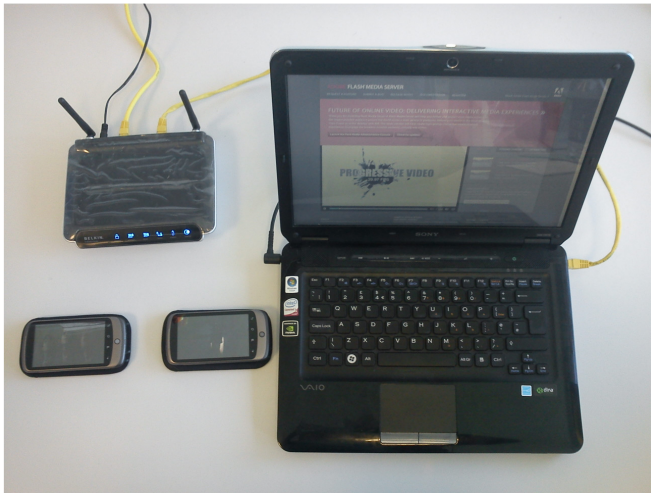
Figure 4 – Test Setup: Server (laptop), Access Point and two Client Devices
