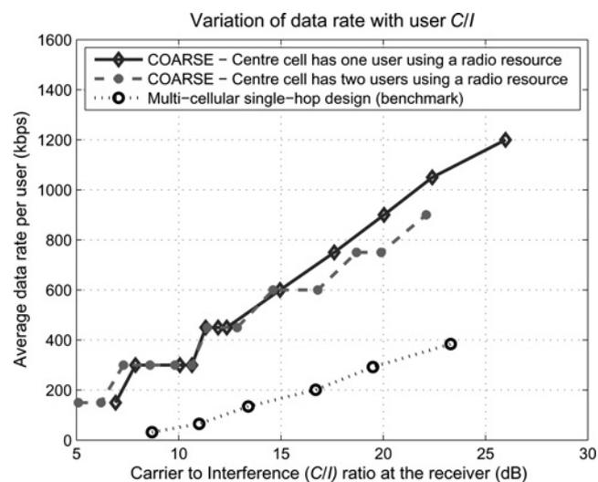
Fig. 5 Variation of data rate per user with carrier-to-interference ratios
