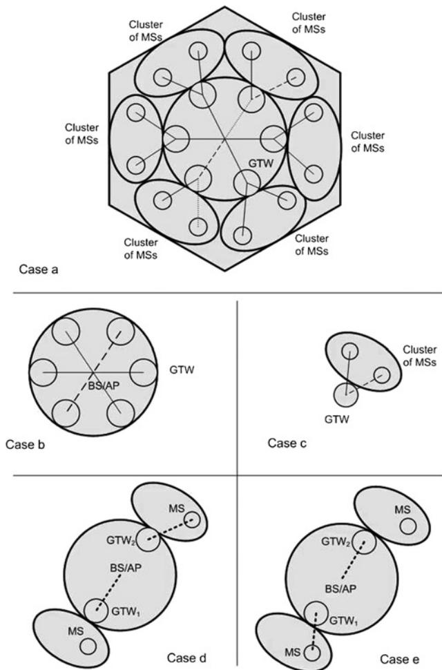
Fig. 1 Two-hop cluster-based cellular architecture
