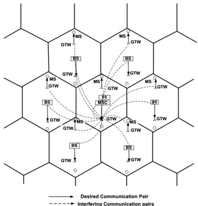
Fig. 2 Interference at the gateway node of centre cell
