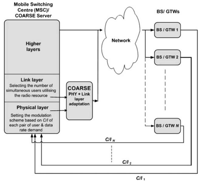
Fig. 4 Cross-layer design at the MSC acting as COARSE server
