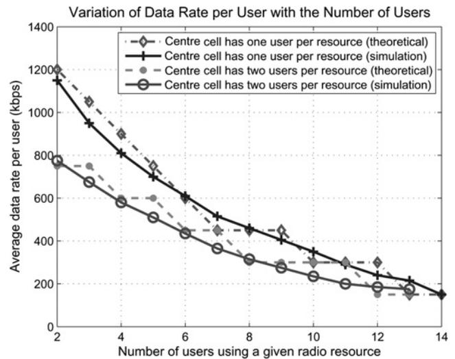
Fig. 6 Variation of data rate per user with varying number of users
