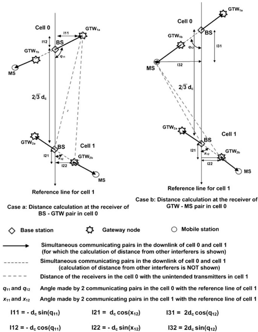
**Fig. 3** Distance calculation at the receivers of BS → GTW and GTW → MS pairs
