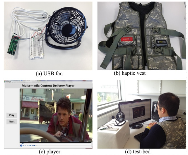
Fig. 2: The equipment and software used in the mulsemedia delivery system employed in the user tests
