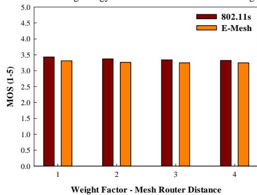
Fig.18. MOS achieved using 802.11s and E-Mesh with variable weights on mesh router distance when the mesh routers are moving
