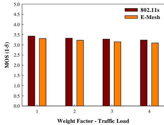
Fig.14. MOS achieved using 802.11s and E-Mesh with variable weights on traffic load when the mesh routers are moving
