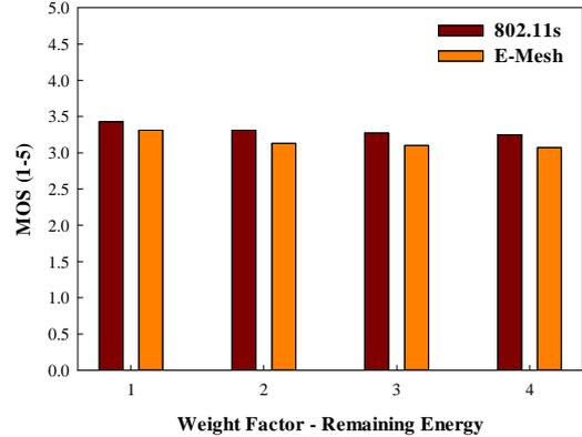
Fig.16. MOS achieved using 802.11s and E-Mesh with variable weights on remaining energy when the mesh routers are moving
