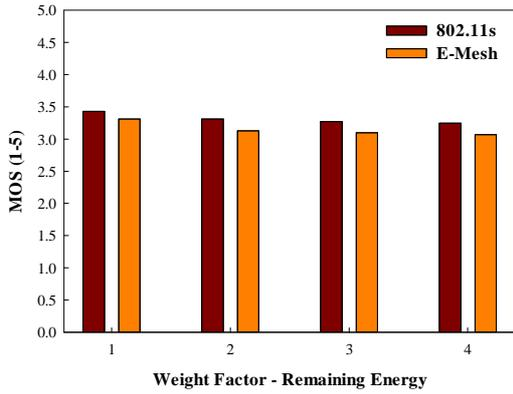
Fig.15. MOS achieved using 802.11s and E-Mesh with variable weights on remaining energy when the mesh routers are static
