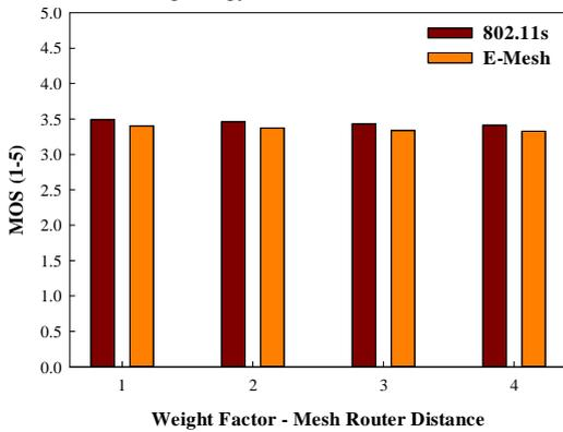
Fig.17. MOS achieved using 802.11s and E-Mesh with variable weights on mesh router distance when the mesh routers are static
