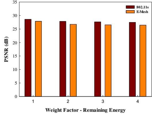
Fig.10. PSNR achieved using 802.11s and E-Mesh with variable weights on remaining energy when the mesh routers are moving
