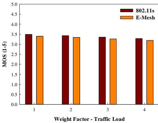
Fig.13. MOS achieved using 802.11s and E-Mesh with variable weights on traffic load when the mesh routers are static
