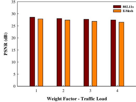
Fig.8. PSNR achieved using 802.11s and E-Mesh with variable weights on traffic load when the mesh routers are moving
