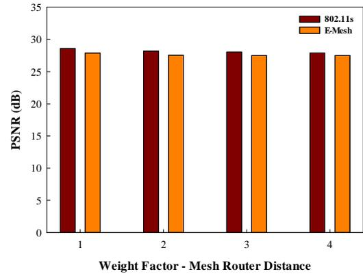
Fig.12. PSNR achieved using 802.11s and E-Mesh with variable weights on mesh router distance when the mesh routers are moving
