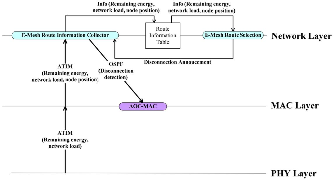
Fig.3. Network/device-condition-based information between different OSI layers
