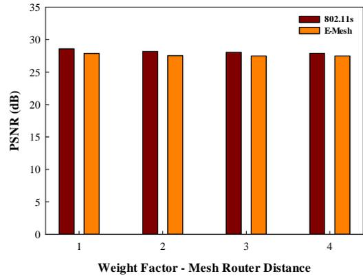
Fig.12. PSNR achieved using 802.11s and E-Mesh with variable weights on mesh router distance when the mesh routers are moving
