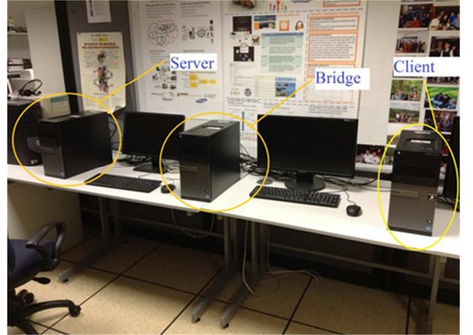
Fig.5. Experimental real-life test-bed topology used - Deployment
