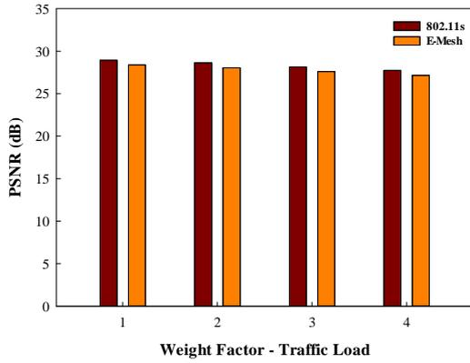
Fig.7. PSNR achieved using 802.11s and E-Mesh with variable weights on traffic load when the mesh routers are static
