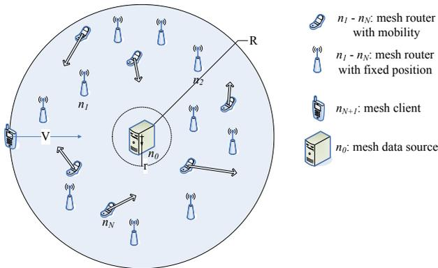
Fig. 1. Wireless mesh network topology
