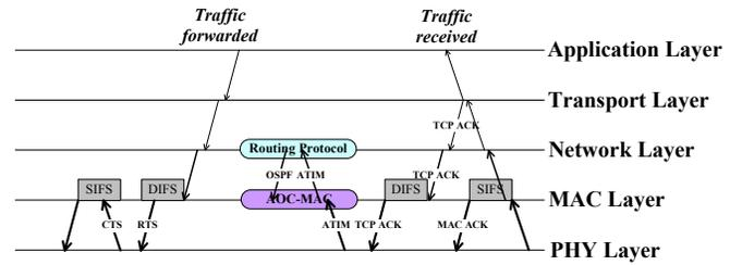
Fig. 3. Network information exchange between different OSI layers
