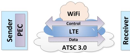
Fig. 3. PEC Framework - Dual Communication Channel Principle.
