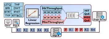
Fig. 9: The deep neural network for QoE prediction: the figure illustrates the operations of the whole predicting process along with generating requests, including collecting client-side information, estimating throughput and predicting QoE gains.
