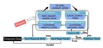
Fig. 11: The correspondence of hooks in ATS: it shows how a request triggers the related actions in ATS which exploits hooks to finish transactions.
