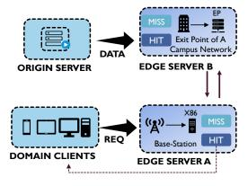
Fig. 5: The cooperative architecture of adjacent edges: each edge serves the covered users with the assistance from the adjacent edge.
