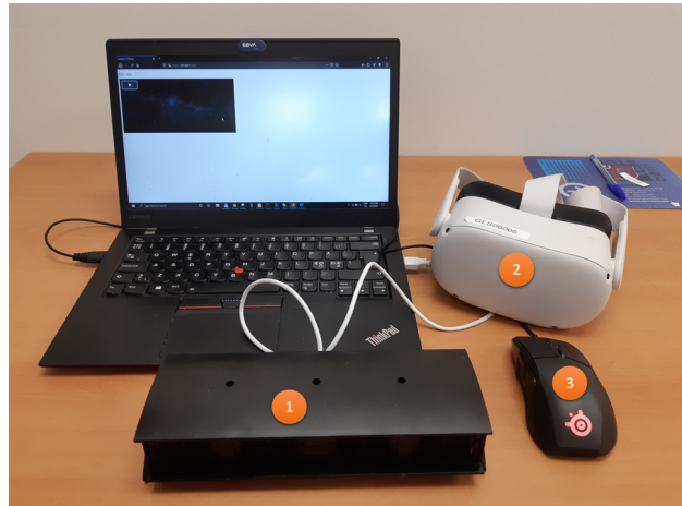
Fig. 1. The prototype of the solution. 1: olfactory machine, 2: Oculus Quest 2 VR headset, 3: haptic mouse
