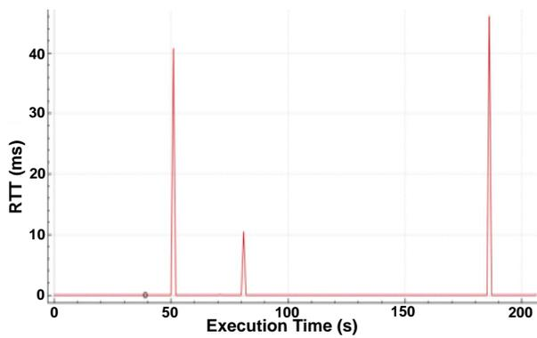
Fig. 7. RTT Between the Application Server and Left Controller PC
