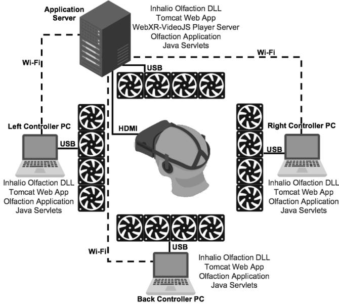
Fig. 5. Testbed Implementation
