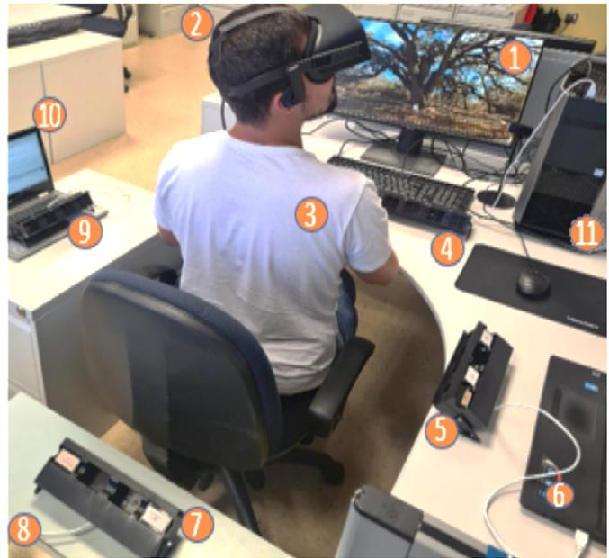
Fig. 1. Real Life Testbed - (1) 360 Video (2) VR Headset (3) User (4) Front Olfaction Dispenser (5) Right Olfaction Dispenser (6) Right Controller PC (7) Back Olfaction Dispenser (8) Back Controller PC (9) Left Olfaction Dispenser (10) Left Controller PC (11) Application Server
