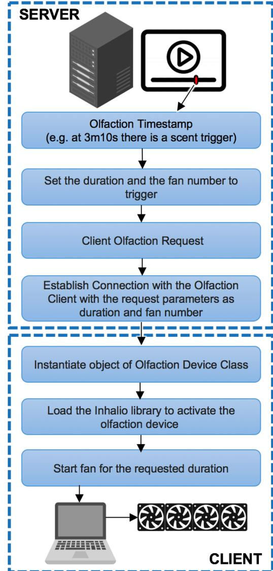
Fig. 3. Olfaction Controller
