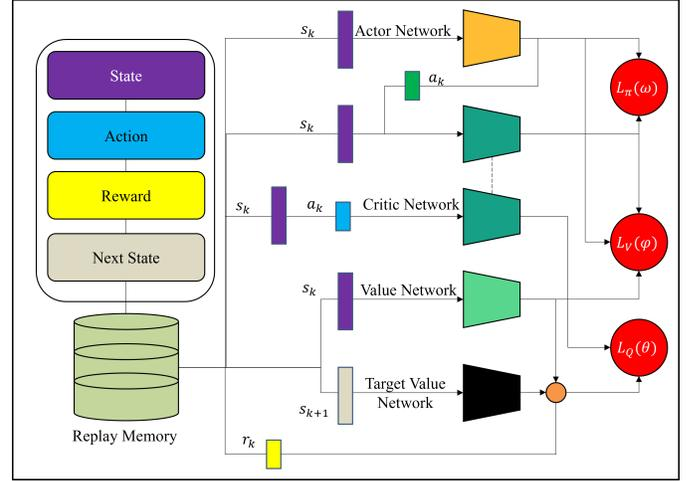
Fig. 5: Training methodology of the proposed I-SAC model. and covariance, which are then used to represent the policy as a Gaussian distribution [22].
