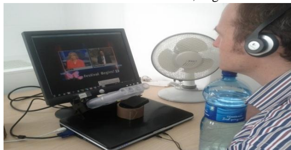
Fig. 1: Olfactory and video media display system [23].
