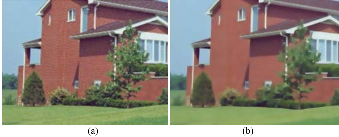
Figure 1. (a) Original natural image. (b) Filtered image resulting after the application of the bilateral filtering. The standard deviation values in the spatial and intensity domain respectively are set to \sigma_d=3 and \sigma_r=20 .
