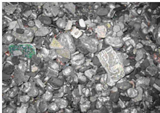
Fig. 1. Fractions of different nonferrous metals and Stainless Steel resulting from the WEEE recycling process.
