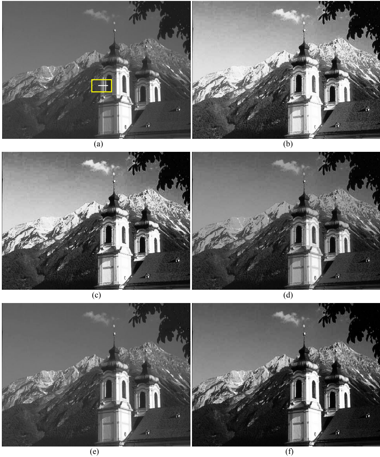
Fig. 10. Contrast enhancement results – Berkeley database [33] image. (a) Input image. (b) GHE. (c) BP-BHE. (d) MMBE-BHE. (e) DHE. (f) Proposed TV-L 1 TE-HE. Note the crisper edge enhancement obtained by the proposed TV-L 1 TE-HE when compared to GHE and other HE-based contrast enhancement strategies (for additional details please refer to Fig. 8).
