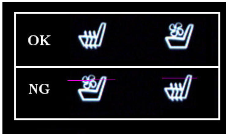
Figure 5.2.5: Seat Heat and Seat Fan Failure Detection
