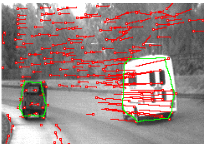
Figure 2-17. The ASSET-2 Tracking algorithm in an unconstrained image sequence. (Image is from the Smith ASSET-2 report (Smith, 1995)).
