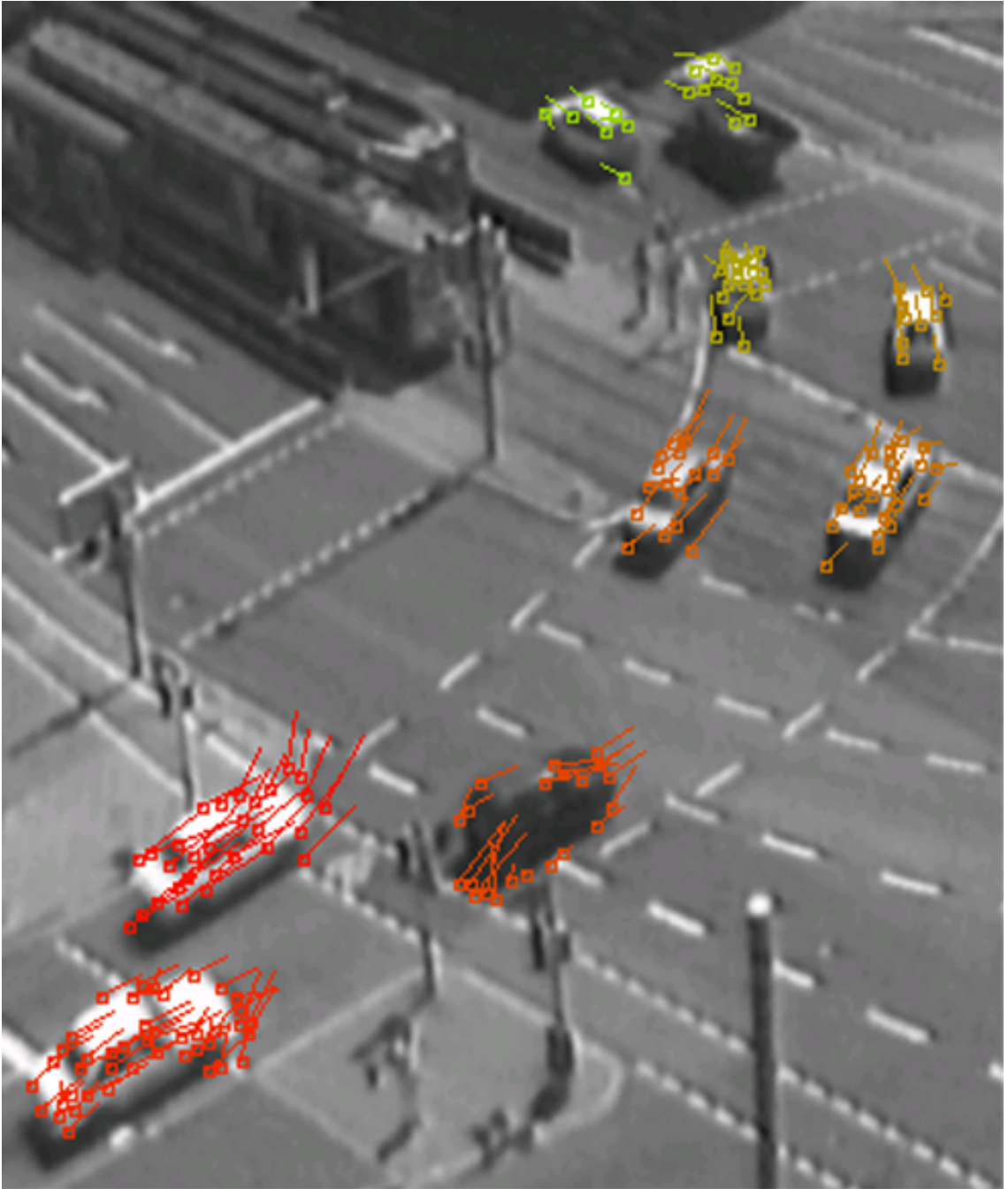
Figure 5-47. The junction results (zoomed by 1.5), with the vector heads located on the position of the objects in the current frame, pointing towards the exact position of that feature in the next frame. Each set of vectors (clustered to mesh) are represented using different colours.
