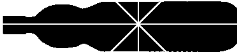
Figure 3.8 Diagram shows a bottle split into eight sections using the radial coding technique.
