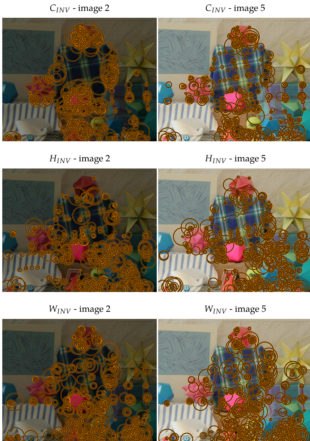
Figure 4.4: Visual illustration of the local feature extraction results on two different imaging conditions of the Moebius set, using three separate gradient types: C_{INV} , H_{INV} and W_{INV} .
