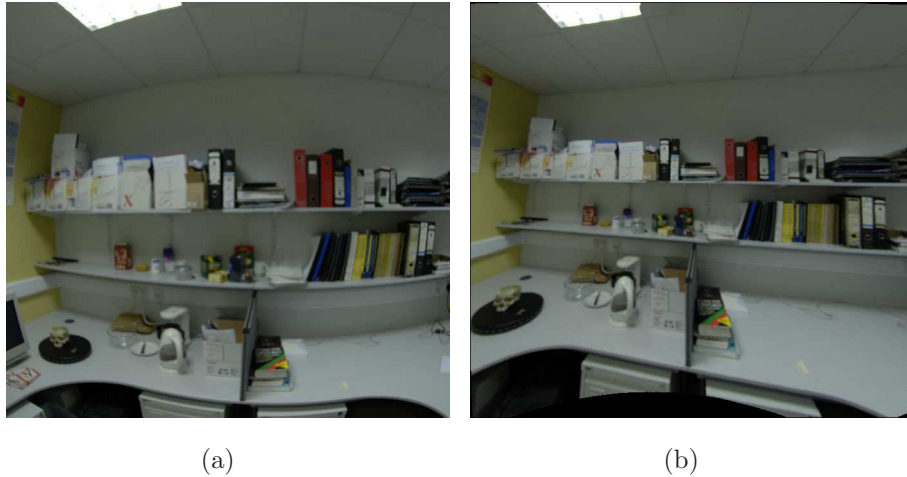
Fig. 3.17: (a) Original fisheye image; (b) Fisheye image after distortion correction using active grids input data.
