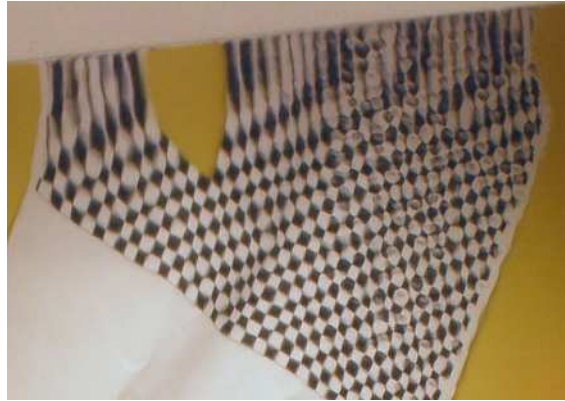
Fig. 5.6: Portion of a flexible mirror image showing aberration in the upper region due to poor mirror quality.
