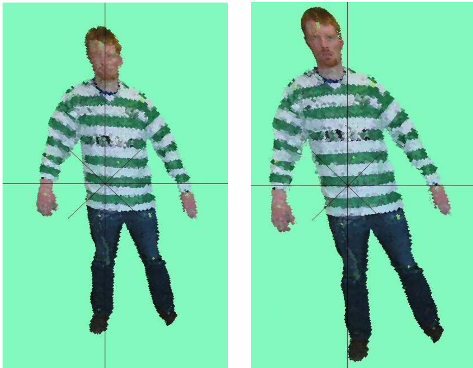
Figure 7.9 Left: the reconstructed human model at resolution r=25 . Right: same 3D model with the face region refined at resolution r=6
