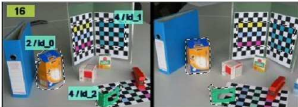
Figure 4.3 a. An example showing two images (out of a sequence of seven) with the regions corresponding to a box, a checkerboard area and a plastic object selected and labeled with the final resolution ( r=6 ). The resolution of the initial reconstruction is the upper left corner ( r=16 ).
