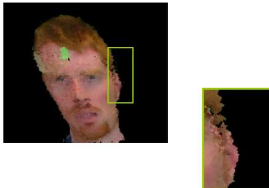
Figure 8.1 Detail of holes in the reconstructed surface, caused by grazing view angles
