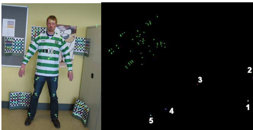
Figure 7.7 Left: A sequence image with the tracked points. Right: The recovered metric structure of the tracked points and the camera positions
