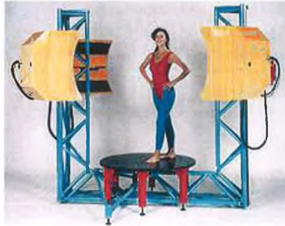
Figure 3.12: The Cybeware whole body scanner system 12 .
