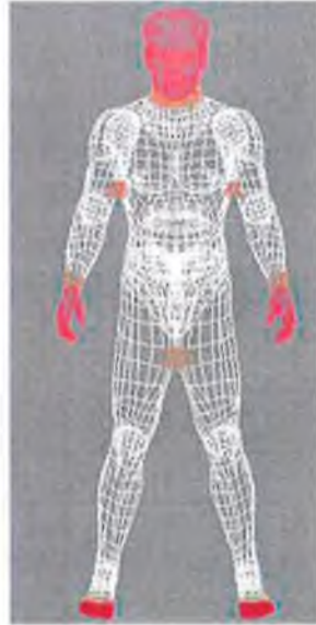
Figure 4.34: Visual marking of the rigidity on the underlying model. The red parts have strong rigidity and tightly bound vertices. The lighter red parts indicate weaker internal forces.
