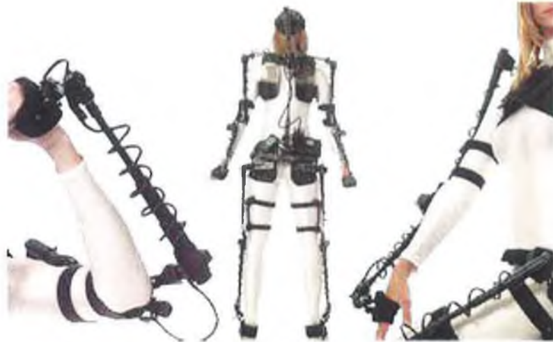
Figure 3.9: The Gypsy Motion capture System is shown. This motion capture system is an electro mechanical system that consist of an exoskeleton made of lightweight aluminium rods that follow the motion of the performer's bones 11 .
