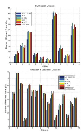
Fig. 2. Feature matching results for the three categories in the dataset. The results show the number of matched points as a percentage to the total keypoints extracted in an image.
