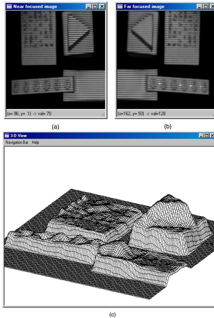
Figure 8. Depth estimation for a scene defined by textureless, textured and mildly specular objects. (a) Near focused image. (b) Far focused image. (c) Recovered depth.
