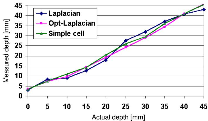
Figure 6. Recovered depth for a randomly textured planar object placed at different elevations from the baseline of the workspace.
