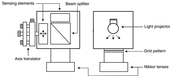
Figure 3. The diagram of the developed range sensor.
