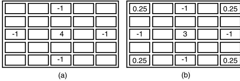
Figure 2. The focus operator. (a) Standard Laplacian. (b) Four peak Laplacian operator.
