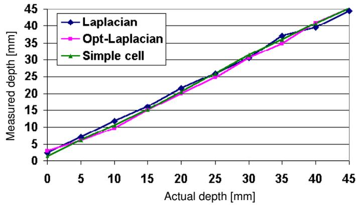
Figure 5. Recovered depth for a textureless planar object placed at different elevations from the baseline of the workspace.
