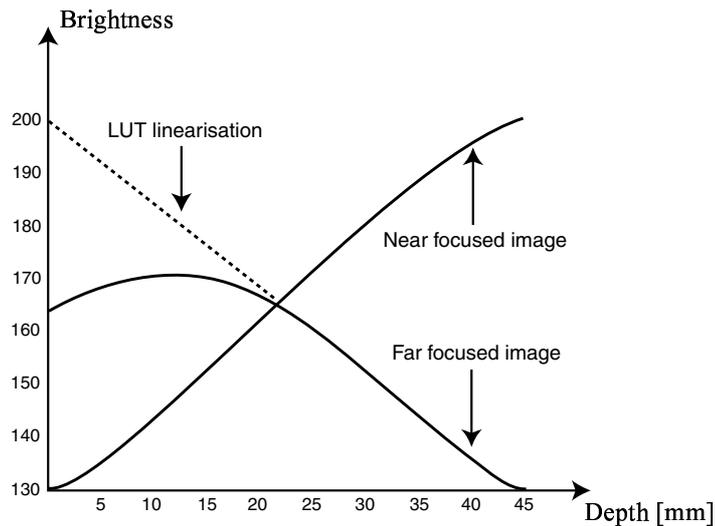
Figure 4. The effect of the supplementary blur introduced by the lens of the light projector. The errors are compensated by using a look-up table (LUT) linearisation. Numerical values are obtained when the simple cell was employed as focus operator.
