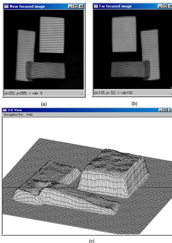
Figure 7. Depth estimation for a scene defined by polyhedral objects. (a) Near focused image. (b) Far focused image. (c) Recovered depth.
