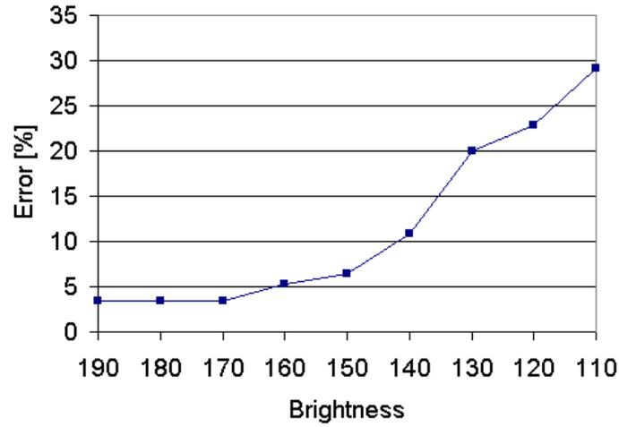
Figure 9. Relation between the depth error and the brightness of the object surface.
