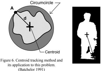
of the region, the velocity of the region and the position of the region. It uses logic and uncertainty weightings to build algorithms to find the best match. This allows objects to be tracked individually in the sequence.
