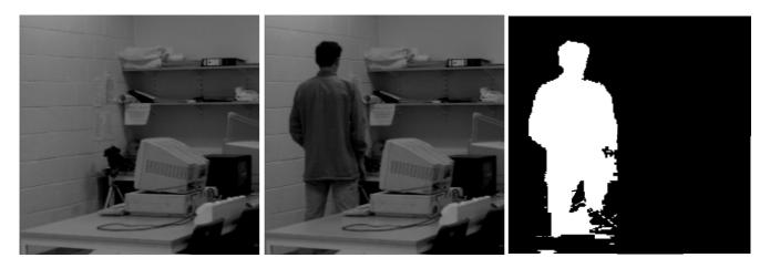
Figure 5. Showing the reference image, the image with the object and the extracted results.
