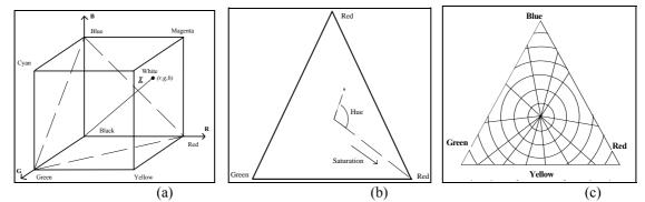
Figure 3.(a) The RGB colour space with an arbitrary colour triplet (r,g,b), (b) Section from the RGB cube showing the relationship of HSI parameters to the RGB colour space, (c) showing a filter used in the segmentation of images based on hue and saturation.
