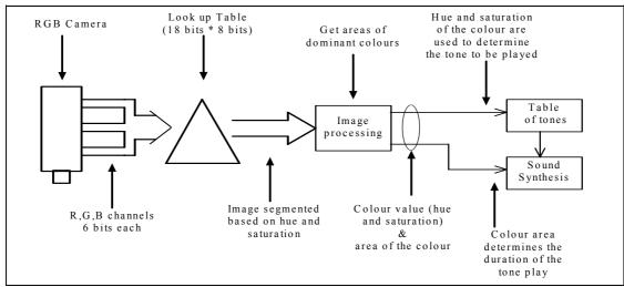
Figure 4. Operation of the Colour to tone converter
