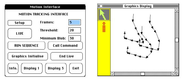
Figure 7. The motion tracker interface and the results display window.
